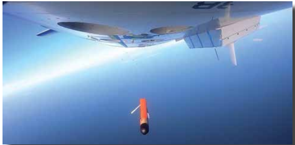
View of the underside of the NOAA Hurricane Hunter plane as the Altius-600 uncrewed aircraft (research drone) is deployed high over a field during flight tests on January 15, 2021.
