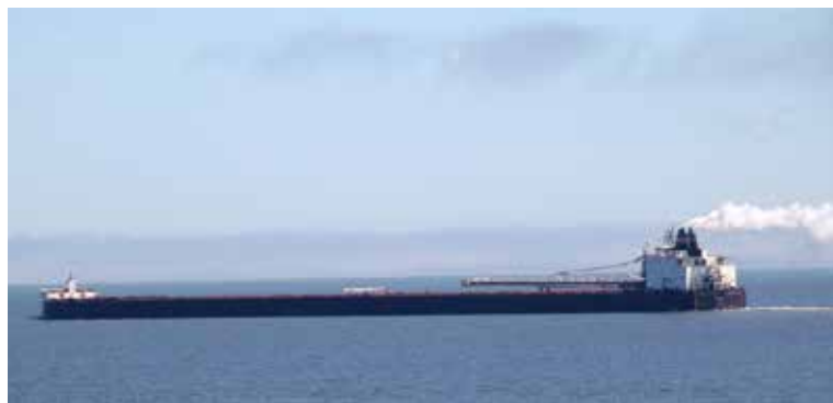
The MV American Spirit, a typical laker with self loading/unloading conveyor belt MIKE TODD, 2017, WOLDHISTORYPICS.COM
