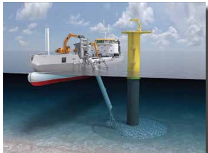
Scour protection after installation of the monopile (shown in gray) and the transition piece (shown in yellow)
